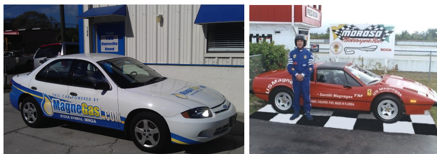
Figure 26: A view in the left of a Ford Cavalier produced to run on compressed natural gas and run on compressed magnegas with no appreciable CO and HC in the exhaust, and a view in the right of a Ferrari 308 GTS 1981 converted to run on compressed magnegas and shown at the Moroso International Race Track, Florida, to be competitive with same Ferraris running on gasoline.
